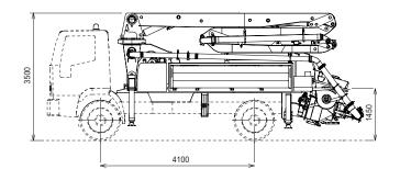
Dimensions varying according to truck assembly
